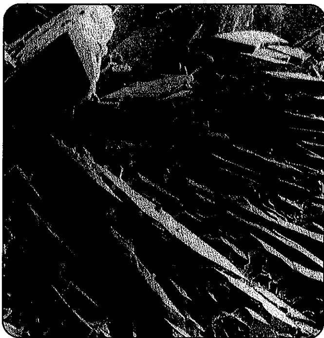
▲ Figure 6 This magnification of a piece of metal shows that even a very smooth surface has tiny high and low areas that cause friction.
